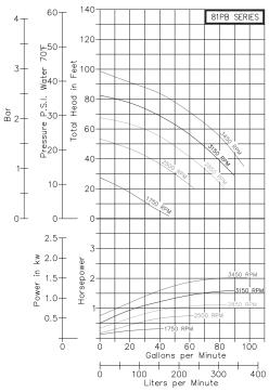
The height of the suction lift should be kept to an absolute minimum and the size of the suction pipe should be equal or larger than the pump inlet port. A foot valve with strainer is recommended a the beginning of the suction line. Self-priming centrifugals must be operated with the shaft in the horizontal position, regular centrifugals may be operated with the shaft horizontal or vertical.
